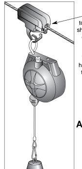
Trolley with hook for tool balancer. Balancer, shown attached, reduces effort by making tools weightless.
