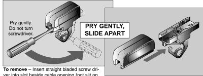
ver into slot beside cable opening (not slit on side of trolley) and pry gently as shown above. Do not turn screwdriver. Slide Apart.
