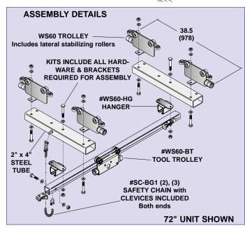
Heavy Duty Rolling Rail mounts in two parallel rails, which must be supported every 6' (1.8m) to maintain rated capacity. Recommended distance between support rails is length of tool rail less 12" (305mm). MAXIMUM RATED CAPACITY OF ROLLING RAIL includes tool, balancer, and attachments.
