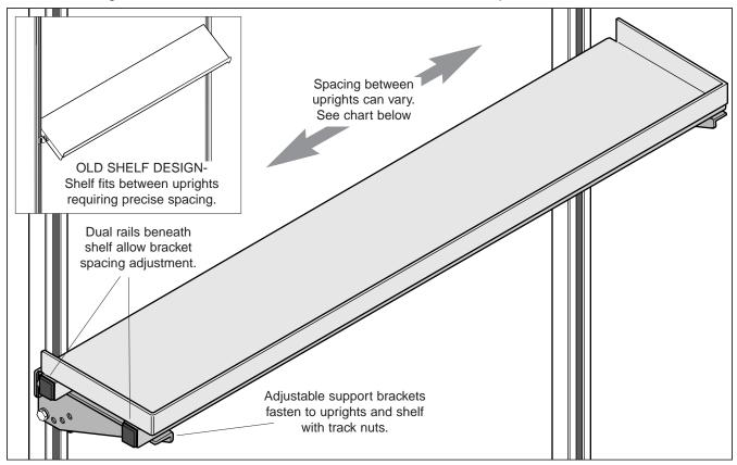
Positive four position shelf tilt (holes, not slots) means shelf attitude can't change because of loose bolts, yet can be easily adjusted to match requirements.
