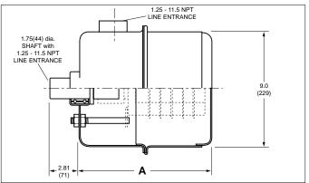
Gleason Slip-Rings may be mounted in virtually any position. Used in Gleason Reels, they are mounted horizontally. Vertical applications include rotating signs and amusement rides. Whichever configuration you choose, it is possible for either the main shaft or the mounting
