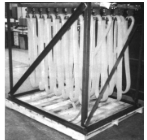
Heavy duty festoon system modified for travel on a curved I-beam. Note two additional saddles on each trolley to handle large number of cables.
