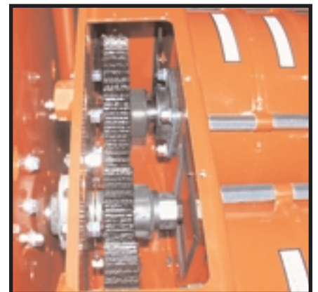
Precision, heavy-duty drive includes convenient detensioning device for de-energizing spring during cable replacement or other maintenance.
