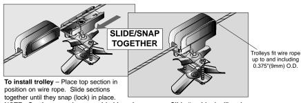
NOTE: Sections may be assembled in only one way. Slide "un-blocked" end into "un-blocked" end. Do not force.
