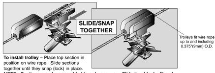
NOTE: Sections may be assembled in only one way. Slide "un-blocked" end into "un-blocked" end. Do not force.
