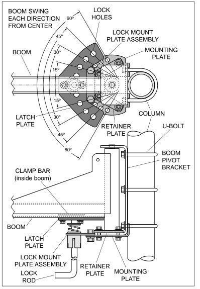
3. Insert bolts with flat washers through clamp plate and mounting plate. NOTE: Bolts go beside, not through, pivot bracket. Secure assembly with nuts, lock washers and flat washers. Make sure mounting plate is properly aligned, with hooks tight against boom pivot bracket. Securely tighten bolts.
