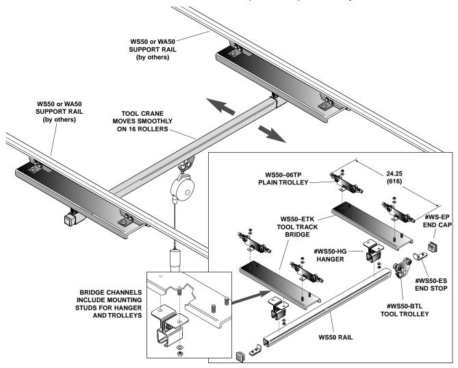
Tool Crane mounts in two WS50 rails. Rails must be parallel and level to allow free travel of crane. Recommended distance between support rails is length of tool rail less 12" (305mm). MAXIMUM RATED CAPACITY OF TOOL CRANE is 50 lbs (22.5 kg) including tool, balancer, and attachments. Unit depth is 24.25" (616mm) bumper–to–bumper.
