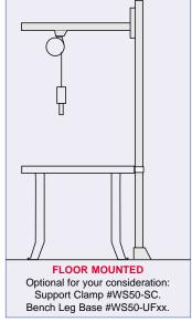
JIB KITS with W3F or W3S prefix include (1) 3' WS30 boom, (1) WS50 vertical column, (1) mounting base, (2) end caps, (1) end stop, (1) balancer trolley, and all hardware. Fixed booms are mounted to the vertical columns with angle brackets, also included.
