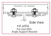
Heavy gauge steel used to mount T-Track sections to support brackets.
