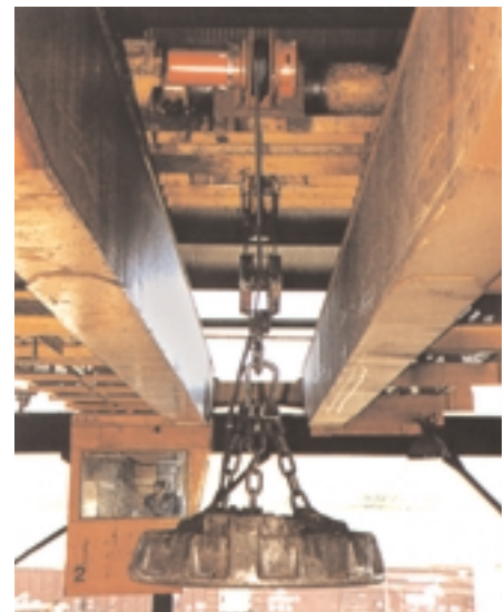
ON THE COVER: Typical Gleason Series "S" reel mounted on an overhead crane for heavy duty, high cycle, vertical lift service.
